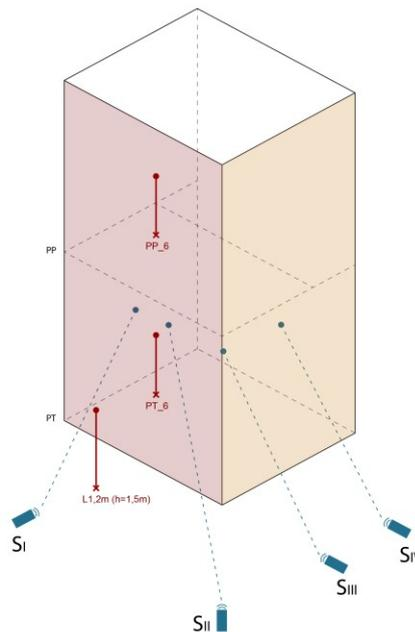
Figure 3 – Scheme of the measurement setup used with indication of the position  $S_I$ ,  $S_{II}$ ,  $S_{III}$ ,  $S_{IV}$  sources.
