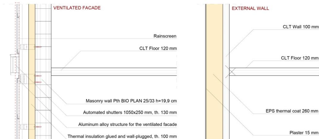
Figure 2 – Construction details: the ventilated façade-floor (left) and external wall-floor junction (right).
