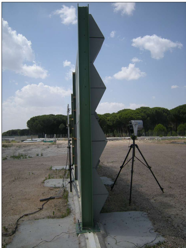
Figure 2. Example of airborne sound insulation measurement in situ .
