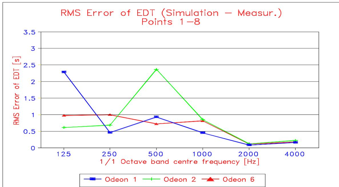
**Fig. 1.** RMS error of the *EDT* prediction as a function of frequency in different *Odeon* runs; same geometric model, different sound absorption values of the plaster (see tab. 1).
