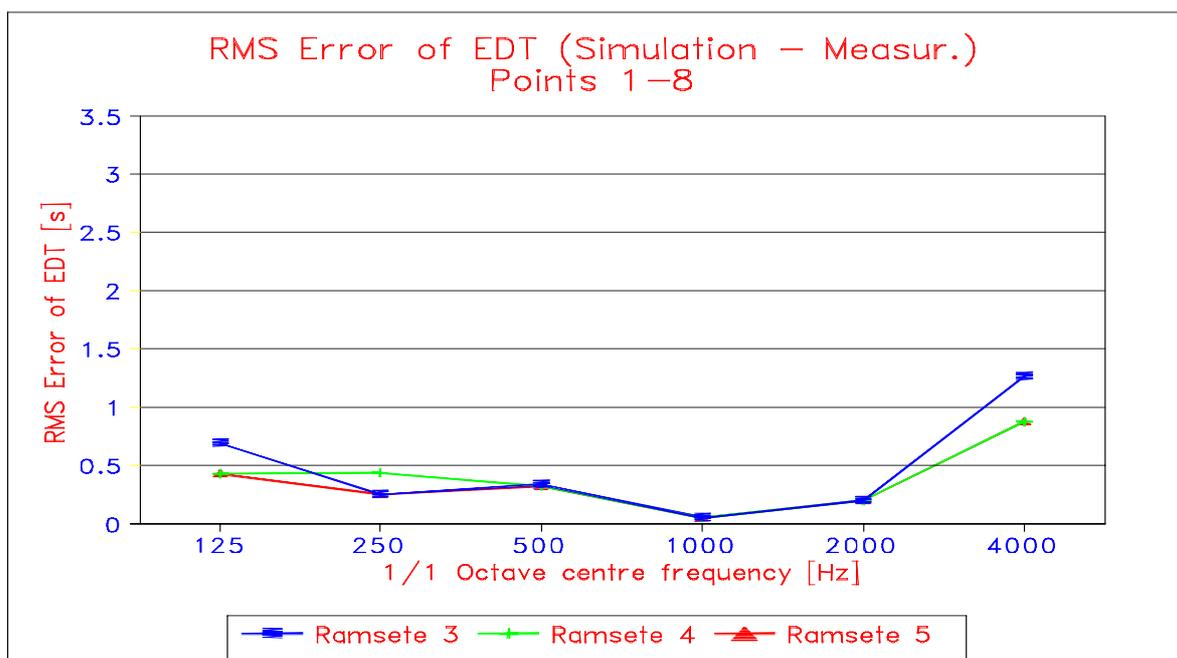
**Fig. 2.** RMS error of the *EDT* prediction as a function of frequency in different *Ramsete* runs; same geometric model, different sound absorption values of the plaster (see tab. 2).
