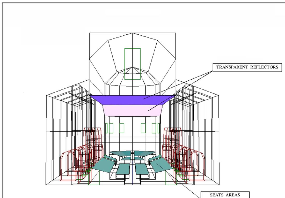
**Fig. 3.** CAD model of the hall with the proposed acoustic corrections as resulted from the *Ramsete* simulation.
