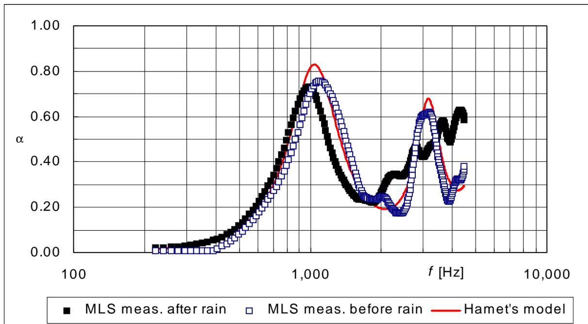
**Figure 3.** Comparison of the narrow band measurement results by DIENCA after rain (black squares) and before rain (empty squares) with the prediction of the Hamet's model ( $s = 40$  mm,  $\Omega = 0.20$ ,  $k_{st} = 2.9$ ,  $\sigma = 47000$  kg/m<sup>3</sup>s) for the same porous layer.
