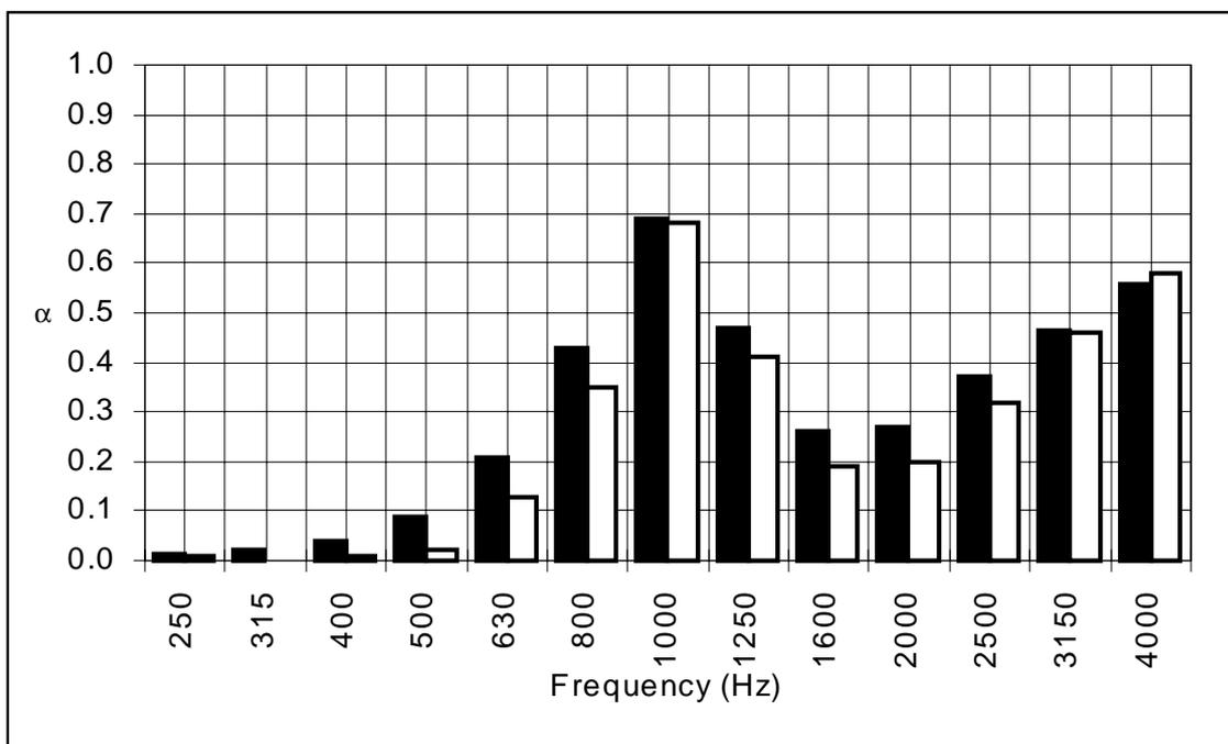
**Figure 2.** Results of the measurements done by DIENCA (black) and LCPC (white) on the same porous asphalt using different test signals and post-processing systems.
