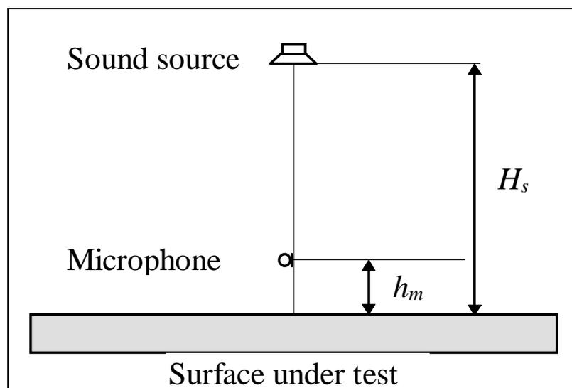
**Figure 1.** Sketch of the measurement set-up.
