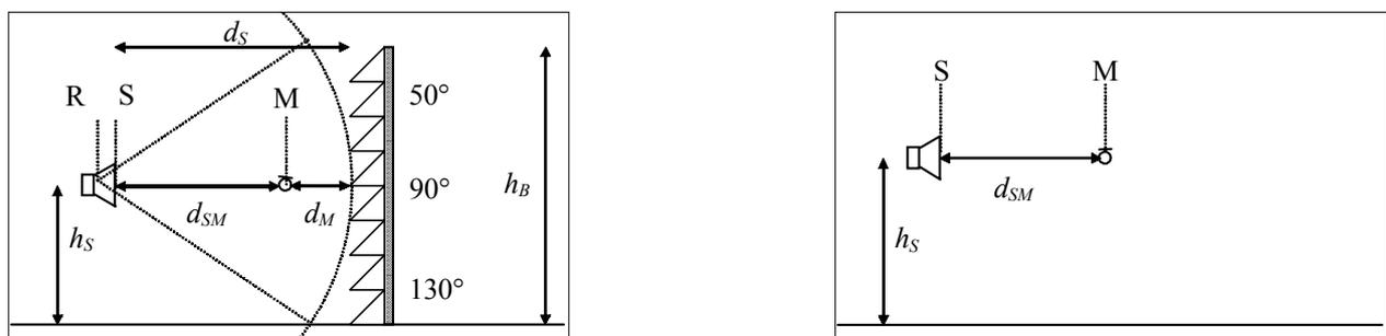
**Figure 1.** Reflection index measurement set-up in front of a non flat noise reducing device: reflected components measurements (left) and “free-field” (incident) component measurement (right).
