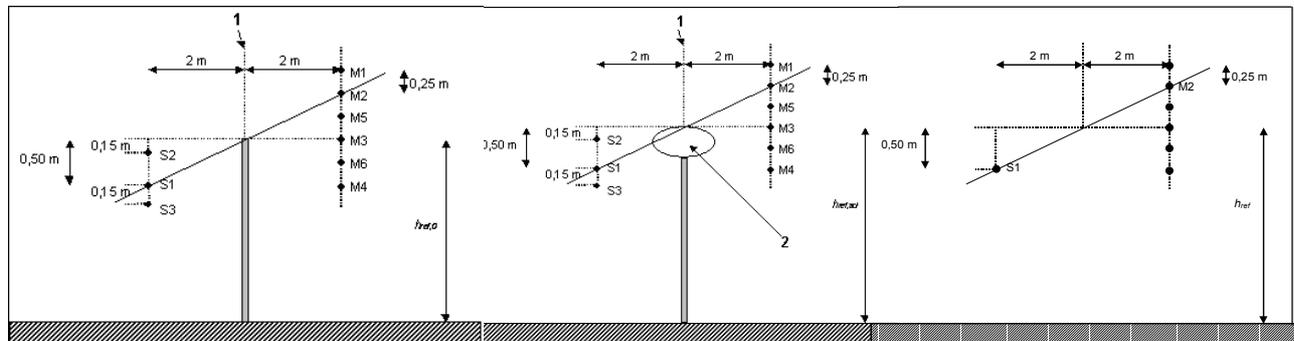
**Figure 3.** Sound diffraction index measurement: loudspeaker (*S*) and microphone (*M*) locations: without added device (left), with added device (centre) and “free-field” (incident) component measurement (right).
