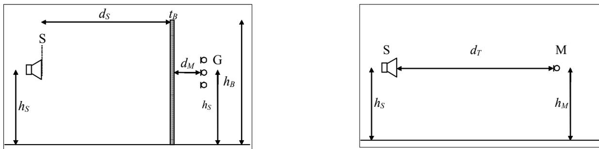
**Figure 2.** *Sound insulation index measurement set-up in front of a non flat noise reducing device: transmitted components measurements (left) and “free-field” (incident) component measurement (right).*
