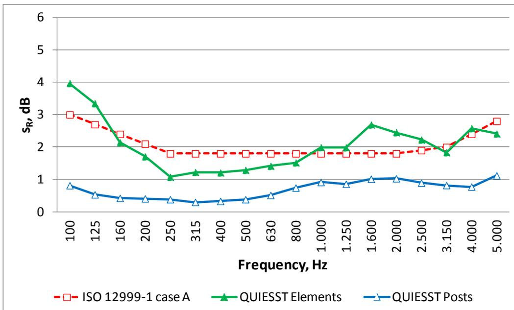
Figure 1 – Standard deviation of measurements in reproducibility conditions
