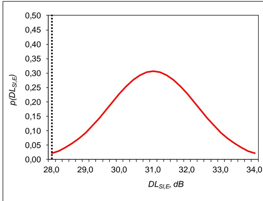
Figure 7 – Example of conformity assessment for the single-number rating of a measurement according to EN 1793-6. The dotted black line indicates the lower tolerance limit of category B3 in situ across acoustic elements: 28 dB. The probability for a measurement result of being less than 28 dB is 1%
