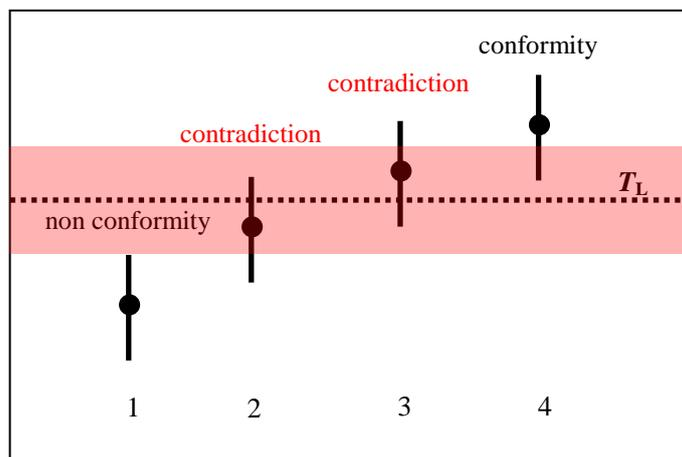
Figure 5 – Sketch of conformity assessment to an lower tolerance limit using both the relaxed guarded acceptance and relaxed rejection rules. The black circle indicates the best estimate of the measurand  $y$  and the black vertical line is the 95% coverage interval  $y \pm U$ . The shaded area is twice the guard band
