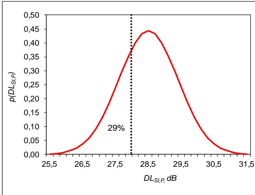
Figure 8 – Example of conformity assessment for the single-number rating of a measurement according to EN 1793-6. The dotted black line indicates the lower tolerance limit of category B3 in situ across posts: 28 dB. The probability for a measurement result of being less than 28 dB is 29%
