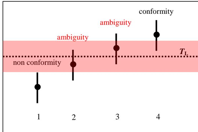
Figure 4 – Sketch of conformity assessment to an lower tolerance limit using both the stringent guarded acceptance and stringent rejection rules. The black circle indicates the best estimate of the measurand  $y$  and the black vertical line is the 95% coverage interval  $y \pm U$ . The shaded area is twice the guard band
