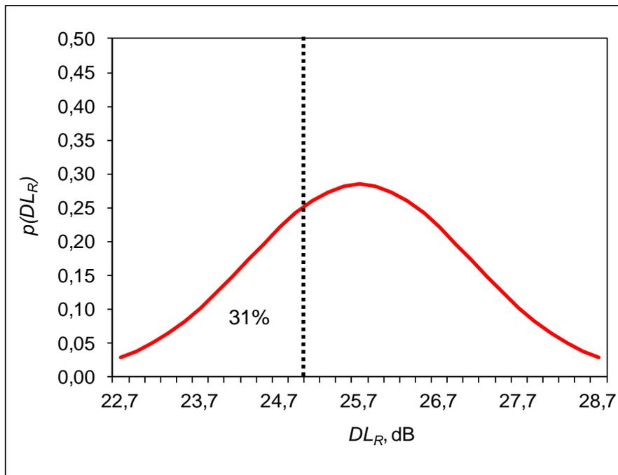
Figure 2 – Example of conformity assessment for the single-number rating of a measurement according to EN 1793-2. The dotted black line indicates the lower tolerance limit of category B3 in a diffuse sound field:
