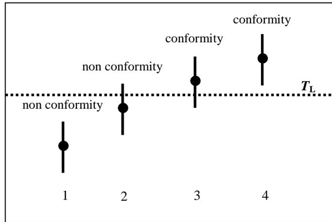
Figure 3 – Sketch of conformity assessment to an lower tolerance limit using the simple acceptance rule. The black circle indicates the best estimate of the measurand  $y$  and the black vertical line is the 95% coverage interval  $y \pm U$
