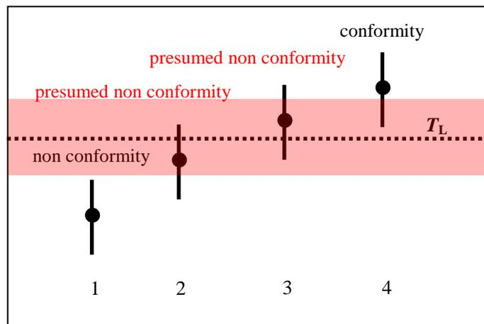
Figure 6 – Sketch of conformity assessment to a lower tolerance limit using the stringent acceptance and relaxed rejection rules. The black circle indicates the best estimate of the measurand  $y$  and the black vertical line is the 95% coverage interval  $y \pm U$ . The shaded area is twice the guard band
