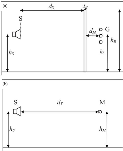
Fig. 6—Sketch of the set-up for the sound insulation index measurement—Normal incidence of sound on the sample—S: loud-speaker front panel—G: measurement grid—M: microphone—(a) transmitted components measurement in front of a flat noise reducing device; (b) free-field (incident) component measurement—( $d_T = d_S + t_B + d_B$ ).
