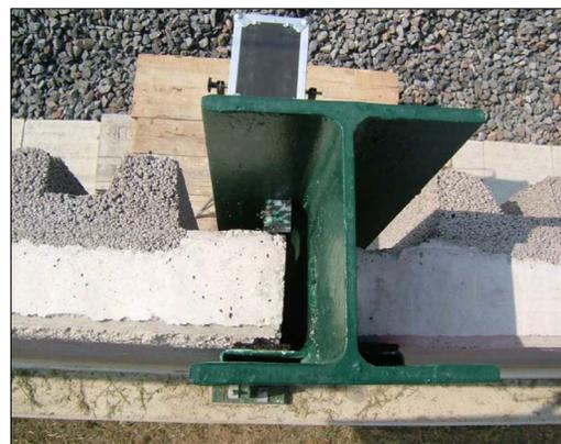
Fig. 19—Top view of the measurement junction between a concrete element and a metallic post. The acoustic leak is clearly visible.
