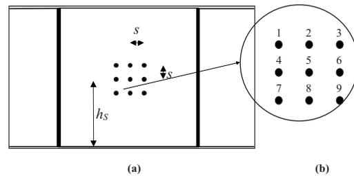
Fig. 5—(not to scale) (a) measurement grid for sound insulation index measurements (front view, receiver side); (b) numbering of the measurement points.
