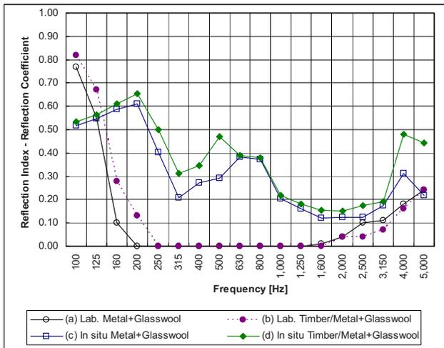
Fig. 10—Reflection coefficient (in the laboratory) and reflection index (in situ) of the metallic cassettes and mixed timber/metal cassettes filled with mineral wool barrier type. (a) in the laboratory, full metal; (b) in the laboratory, mixed timber/metal; (c) in situ, full metal; (d) in situ, mixed timber/metal.
