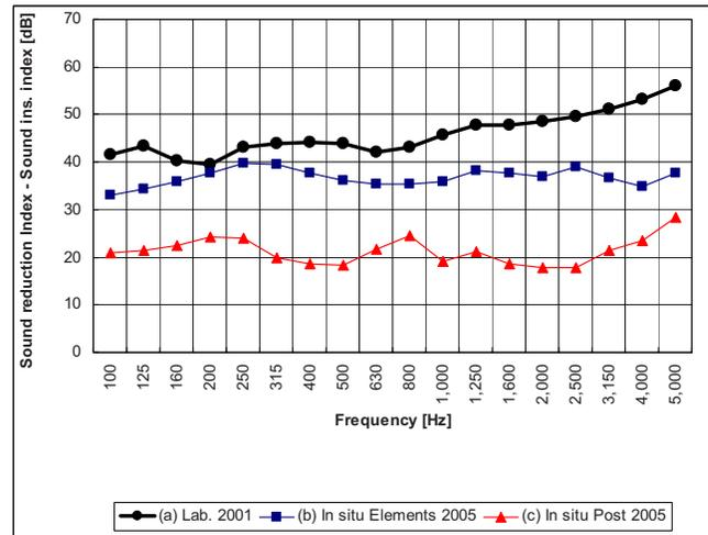
Fig. 18—Concrete barrier: (a) sound reduction index measured in the laboratory; (b) sound insulation index measured in situ in front of the concrete elements; (c) sound insulation index measured in situ in front of a post.
