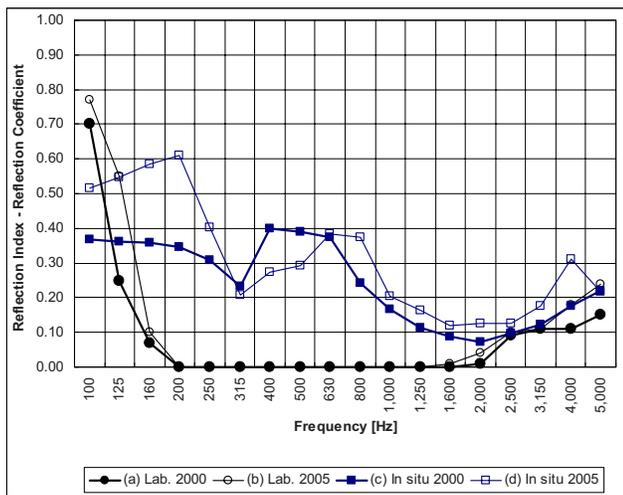
Fig. 9—Reflection coefficient (in the laboratory) and reflection index (in situ) of the metallic cassettes filled with mineral wool barrier type. (a) in the laboratory, filled with rock wool; (b) in the laboratory, filled with glass wool; (c) in situ, filled with rock wool; (d) in situ, filled with glass wool.
