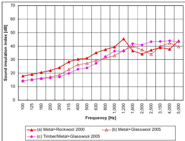
Fig. 14—Sound insulation index measured in situ in front of a post where the junction between acoustic and structural elements has a great influence: (a) full metal filled with rock wool, measured in the year 2000; (b) full metal filled with glass wool, measured in the year 2005; (c) mixed timber/metal filled with glass wool, measured in the year 2005.
