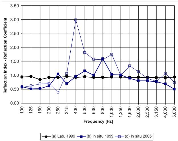
Fig. 12—Reflection coefficient (in the laboratory) and reflection index (in situ) of the acrylic panels barrier type. (a) in the laboratory, measured in 1999; (b) in situ, measured in 1999; (c) in situ, measured in 2005.
