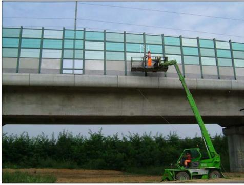
Fig. 2—Placing the microphone grid for airborne sound insulation measurements outside a viaduct.
