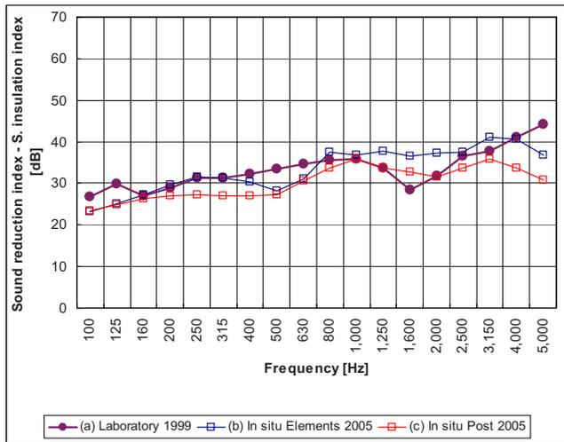
Fig. 20—Acrylic and concrete barrier: (a) sound reduction index measured in the laboratory; (b) sound insulation index measured in situ in front of the acrylic elements; (c) sound insulation index measured in situ in front a post.
