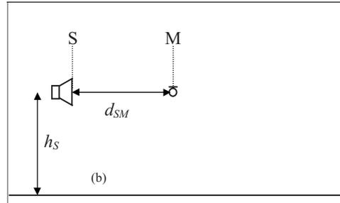
Fig. 4—Sketch of the set-up for the reflection index measurement (example for rotation in vertical direction)—*R*: axis of rotation—*S*: loudspeaker front panel—*M*: microphone. (a) reflected sound measurements, from 50° to 130° in step of 10° on the same rotation plane, in front of a non flat noise reducing device; (b): reference “free-field” sound measurement.
