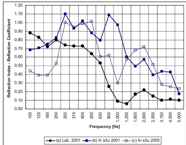
Fig. 11—Reflection coefficient (in the laboratory) and reflection index (in situ) of the concrete panels barrier type. (a) in the laboratory, measured in 2001; (b) in situ, measured in 2001; (c) in situ, measured in 2005.
