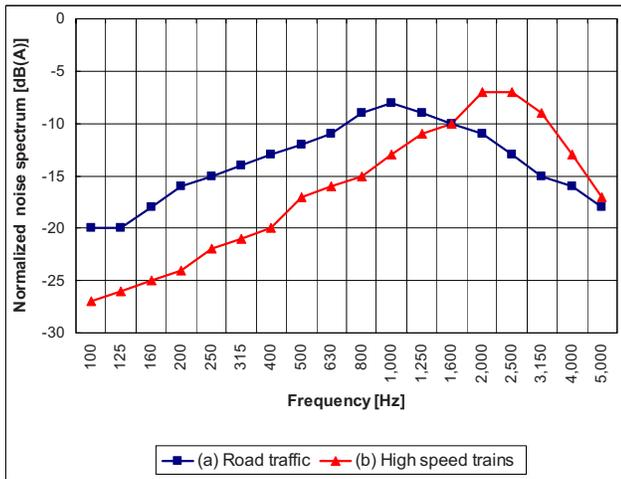
Fig. 7—Reference noise spectra for: (a) road traffic, according to EN 1793-3; (b) high speed railway traffic, according to UNI 11160.
